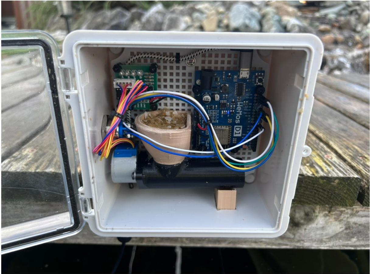
Ensure that there is a hole cut for the food to dispense. Place the box in a location with a good WiFi signal. The project box in the example has a pegboard back that allows for easy mounting of components.
